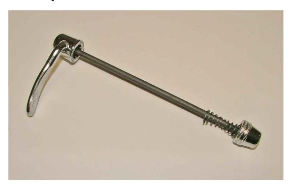
This is the quick-release we ship with CompuTrainer. Most quick-releases shipping today with bike will have levers on the side or on the end and some may even be very large where they meet the body of the quick-release. Our quick-release is a tried and true training stand quick-release almost any bike shop should carry.
