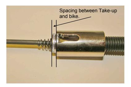
Make sure the threaded end of the quick-release isn't so small that our take-up can contact the bike frame drop-out. The end of or take-up should only contact the quick-release and never the bike frame. If it does, this end of the quick-release is too small for the inside diameter of our take-up. Essentially, you should always see some portion of the quick-release between our take-up and the bike drop-out.
