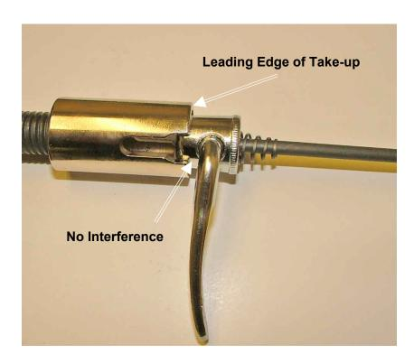
A close-up of the lever into our take-up. The slot is there to allow some quick-releases to be used (as long as it fits into the slot and doesn't hit, or bottom out). There should be no contact with the lever and the leading edge of the take-up.
