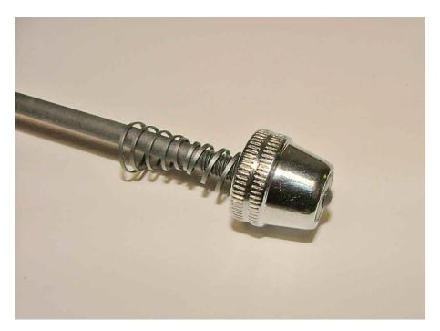
This end can be rounded or squared off, but it should not be plastic (as many are) and should not have finger indents to act as like a thumb-screw. It should be round and symmetrical.
