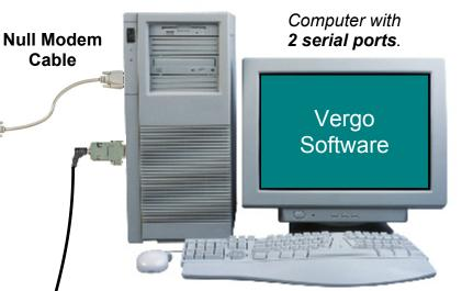
The following diagram is connecting a **Velotron** to a metabolic cart using two computers. Each device and cable connection will still require their own serial port.
